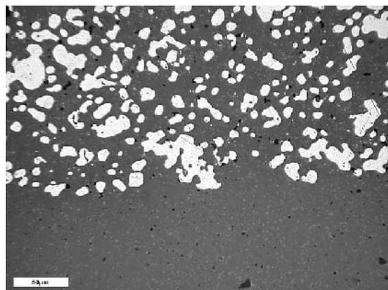
**Figure 5:** Joining zone ceramic - cermet
