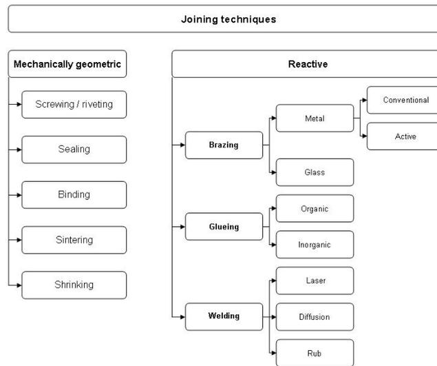
Figure 2: Joining techniques
