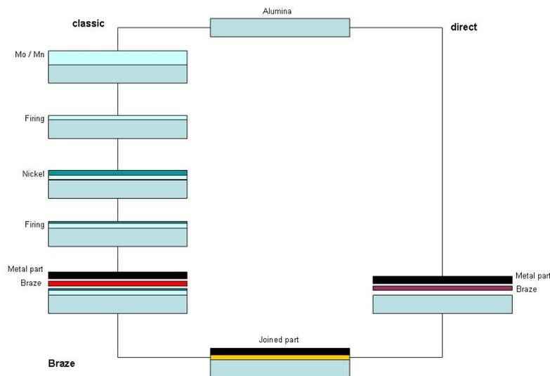
Figure 3: Joining techniques for conventional and active brazing of  $Al_2O_3$  ceramic to metal
