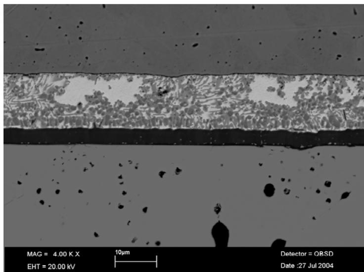
**Figure 5:** Cross-section of active brazed  $\text{ZrO}_2$  ceramic
