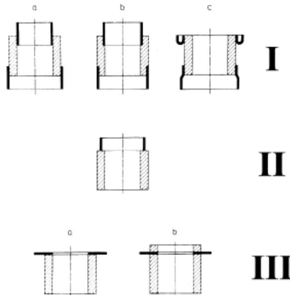
**Figure 7:** Basic types of joints constructions
